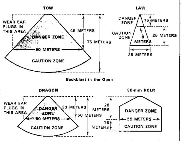
In urban areas, the backblast hezard may be increased by the presence of rubble and the channeling effect caused by narrow streets and alleys. Therefore, friendly troops must be behind protective cover and wear helmets, flack vests, and ear-plugs if they cannot move out of the caution area.
